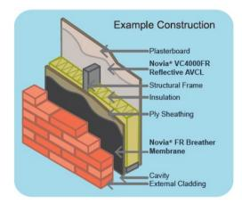
We recommend the use of Novia® 30mm wide Double-Sided Butyl tape1 and Novia® 96mm wide BS 476 Cold Weather Aluminium Foil Lap Tape. In addition, Novia® Airseal 310 FR AVCL sealant can be used in all applications where additional sealing is required, for example internal corners, floor sections or window reveals. See individual tape and sealant datasheets for further product specific information\*.
