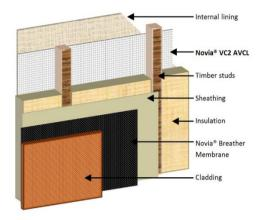
Novia® membranes will only perform their job if they are correctly installed using Novia® tapes as part of a system. Novia® uses a two-tape sealing system on all of our VCL products. It is essential that Novia® membranes are installed correctly using our tapes, otherwise these products will not provide the necessary building design outcomes. One of the major causes of condensation problems within finished buildings is due to poorly installed membranes and where incorrect tapes have been used.
