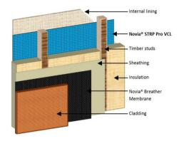
Novia® membranes will only perform their job if they are correctly installed using Novia® tapes as part of a system. Novia® uses a two-tape sealing system on all of our VCL products. It is essential that Novia® membranes are installed correctly using our tapes, otherwise these products will not provide the necessary building design outcomes. One of the major causes of condensation problems within finished buildings is due to poorly installed membranes and where incorrect tapes have been used.
