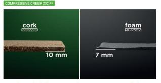
Result: cork delivers superior performance and shows almost the same thickness after being compressed. Less than 10% of thickness loss.
